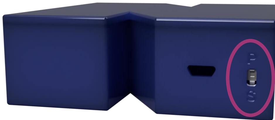
Figure 3: MMBT-S Runtime Mode Switch
